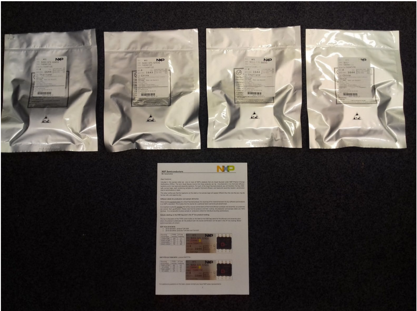
Figure 5: Content of any Quad Source sample shipment: four ESD-safe bags, each containing samples of one of the four sourcing combinations, and a letter explaining by reference to the sample bag labels which samples are from which source.
